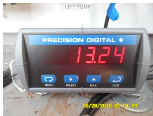
Figure 6. Banner Sensor Reading at ending of evaporation test = 13.24”.
