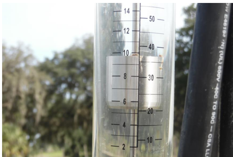
Figure 1. Hydronix Flow Meter rate set at 10GPM.
