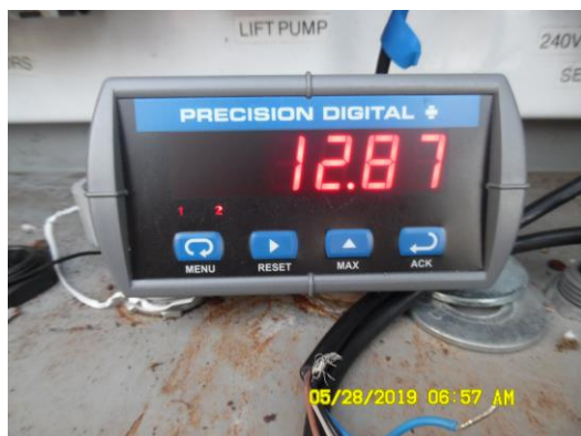
Figure 5. Banner Sensor Reading at beginning of evaporation test = 12.87”.
